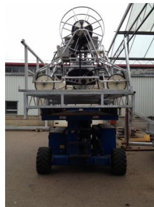
Img. 26 Roof cleaner on scissor lift
